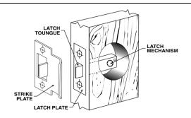
3. Trace latch plate on door, then chisel out from the edge of the door for the latch plate. Insert the latch and attach plate firmly with two flat head wood screws provided. On the door jamb mark the height and the vertical line exactly opposite from the latch tongue for the strike plate.
