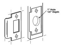
4. Trace hole on the strike plate. Cut out the area on the door jamb directly behind the hole on the strike plate to a depth of about 1/2". This will allow the latch tongue to release inside the strike plate. Attach the plate firmly with two flat head wood screws provided.
